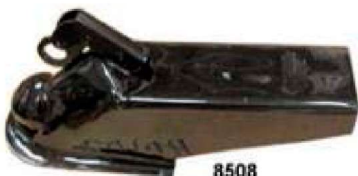
8508 8508 ; HEAVY DUTY TRAILER COUPLER 3" Channel x 2-5/16" Ball, Black Colour, 8500LBS
