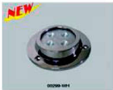
Surface Mount Under Water Light 00099-WH Made of Stainless Steel, with 4x 3W High Power White LEDs, 1.5M. Wire: 85mm Dia., 20mm (Thickness), Quick and Simple to Fit, You Have To Be Fixed On The Transom At The Lowest Possible Location About 2" Above The Bottom of The Boat. Make Sure The Inside of The Transom is Clear. 00099-BU with 4x 3W High Power Blue LEDs
