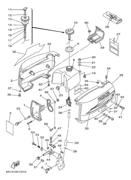
FIG. 1 COWLING . FUEL
