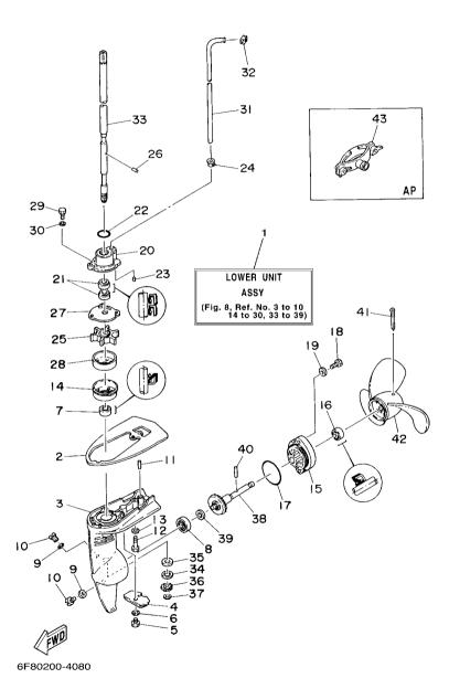
FIG. 8 LOWER CASING. DRIVE
