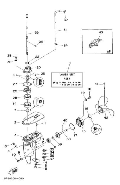
FIG. 8 LOWER CASING. DRIVE
