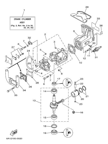
FIG. 2 CYLINDER. CRANKCASE
