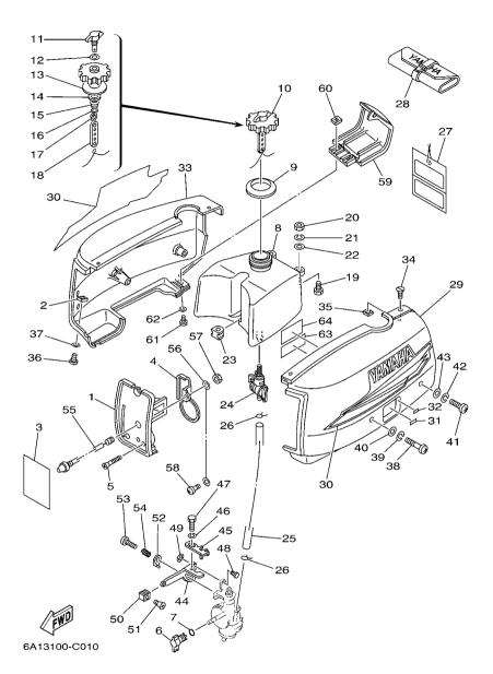
FIG. 1 COWLING . FUEL
