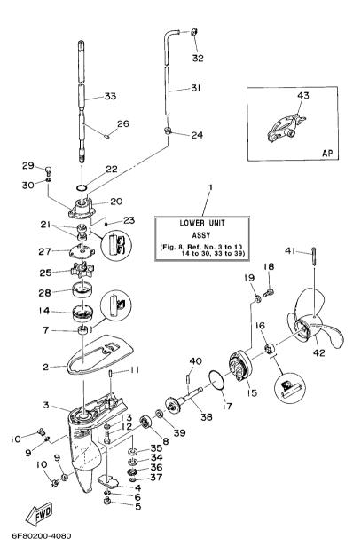
FIG. 8 LOWER CASING & DRIVE
