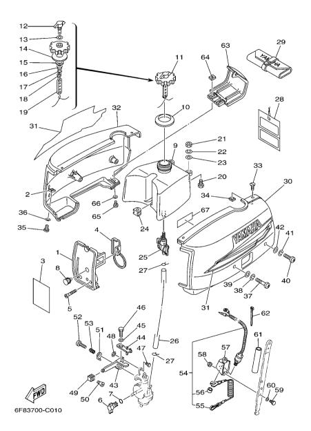
FIG. 1 COWLING & FUEL
