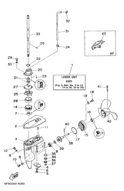
FIG. 8 LOWER CASING & DRIVE
