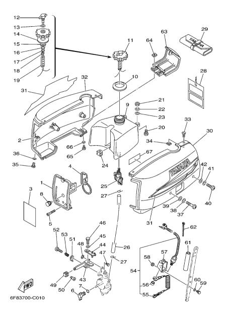
FIG. 1 COWLING & FUEL
