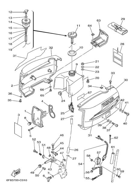
FIG. 1 COWLING & FUEL
