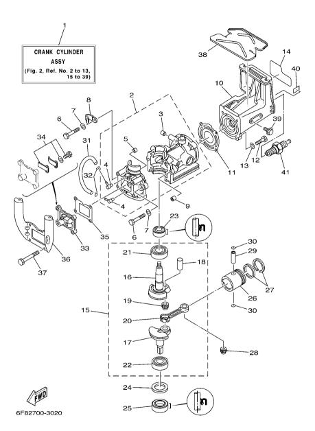
FIG. 2 CYLINDER & CRANKCASE
