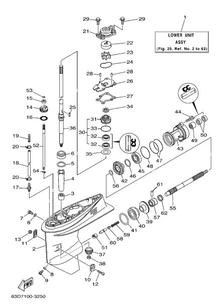
FIG. 25 LOWER CASING & DRIVE 1
