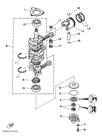
FIG. 3 CRANKSHAFT & PISTON
