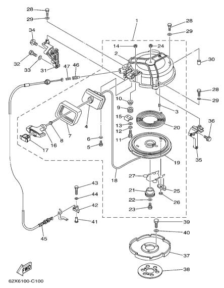
\*1:CUT FROM 50M ROLLS,PART NO.90890-44373,CUTTING LENGTH 2.095M
