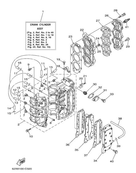
FIG. 2 CYLINDER & CRANKCASE
