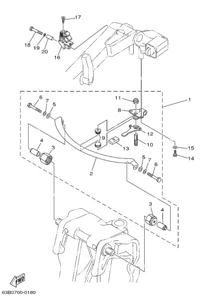
FIG. 18 STEERING FRICTION
