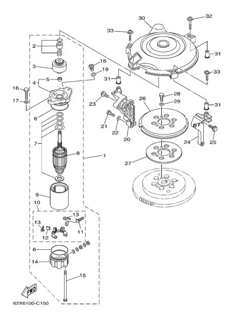
FIG. 12 STARTING MOTOR
