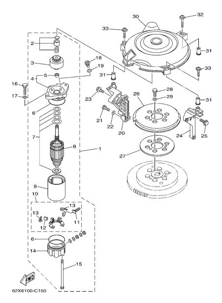
FIG. 12 STARTING MOTOR
