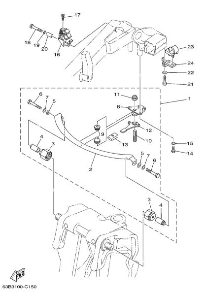
FIG. 15 STEERING FRICTION
