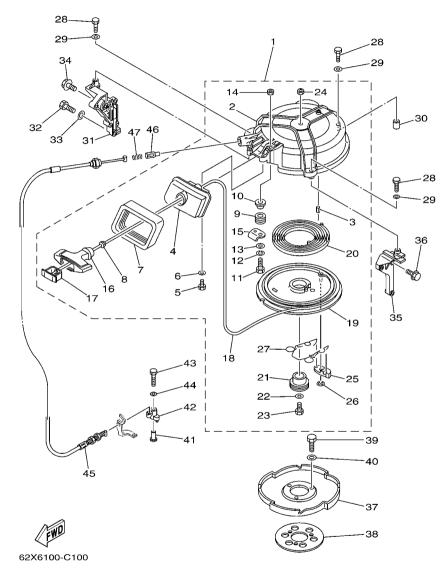
\*1:CUT FROM 50M ROLLS,PART NO.90890-44373,CUTTING LENGTH 2.095M
