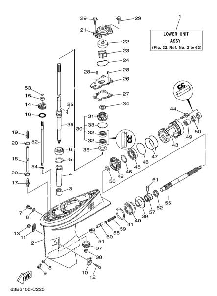
FIG. 22 LOWER CASING & DRIVE 1
