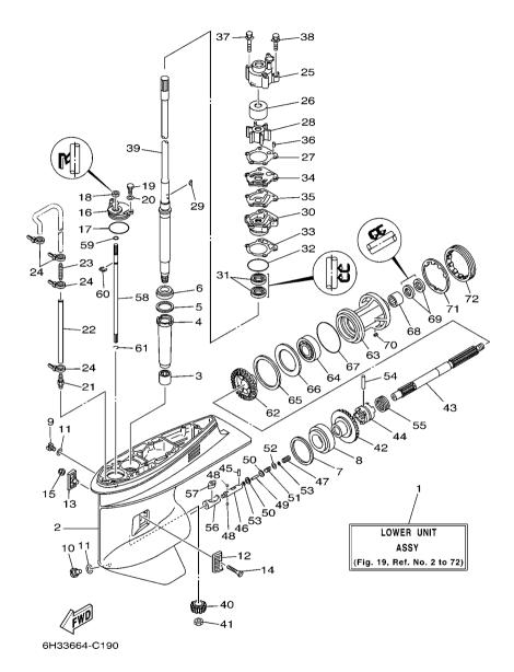
FIG. 19 LOWER CASING & DRIVE 1
