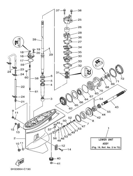
FIG. 19 LOWER CASING & DRIVE 1
