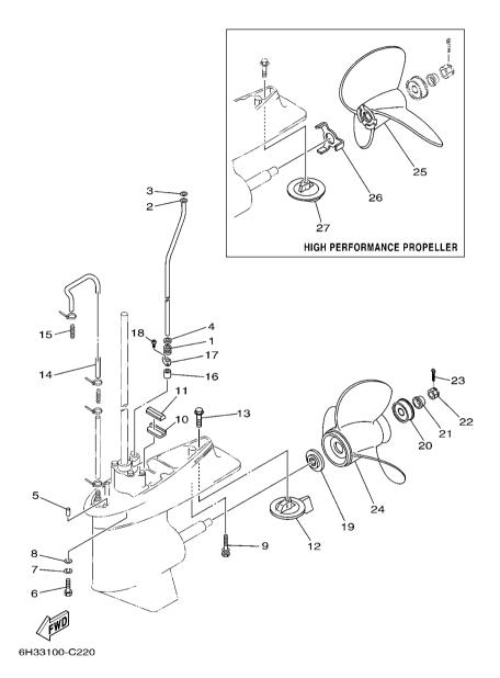
FIG. 20 LOWER CASING & DRIVE 2
