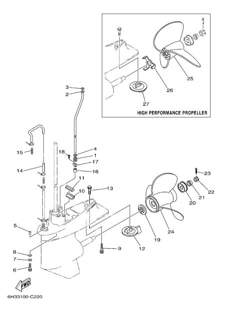
FIG. 20 LOWER CASING & DRIVE 2
