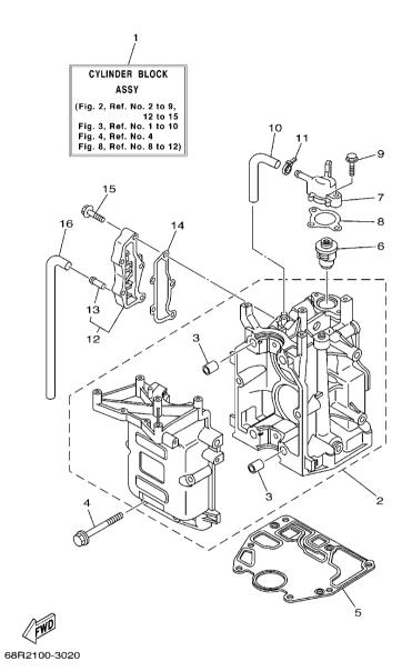
FIG. 2 CYLINDER, CRANKCASE 1
