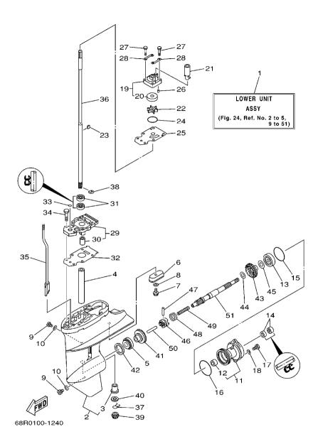
FIG. 24 LOWER CASING. DRIVE 1
